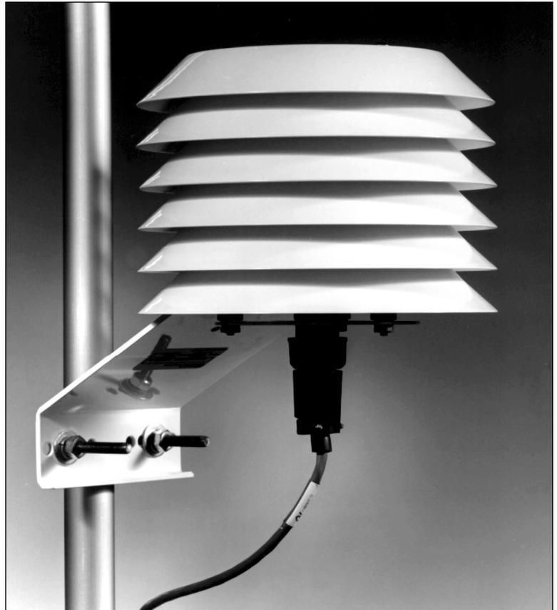
The Model 5980 Naturally Aspirated Radiation Shield is used in remote areas, where power is not available.
