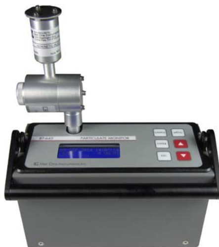
BT-645 w/SCC-112 PM2.5 Sharp Cut Cyclone
