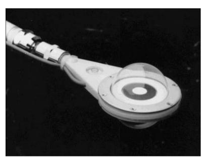
The Model 097 Pyranometer
