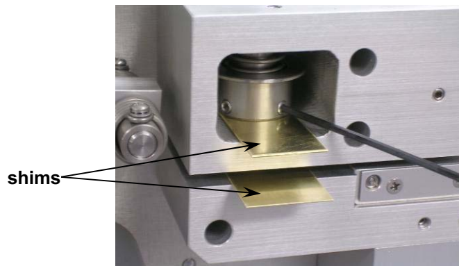
Adjusting the spring tension and nozzle
