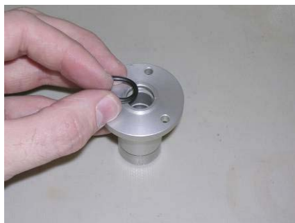
Replacing the nozzle o-ring
