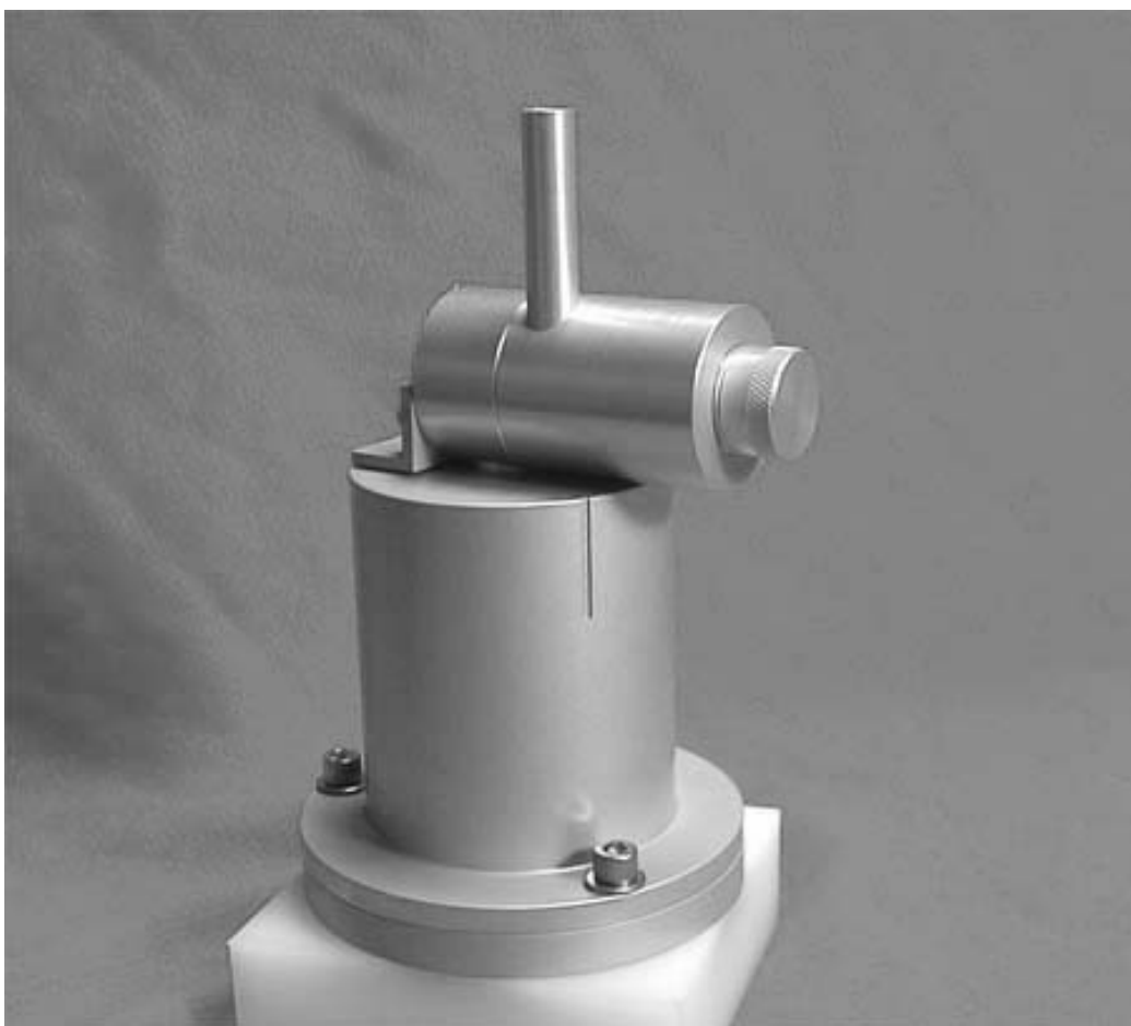
Figure 1.6. View of the Sharp cut cyclone Inlet that provides the PM 2.5 cut-point. Canister is shown Inverted in Canister Assembly Block
