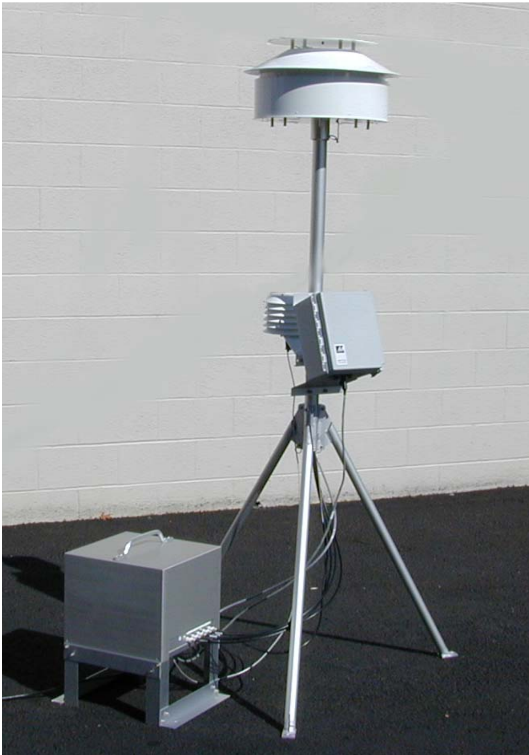
Figure 1.1. SASS showing aspirated Solar radiation shield, Canister Inlets, Tripod, Control Box, and Vacuum Pump Box.
