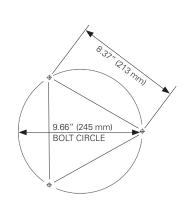
HOLE PATTERN IN BASE FOR 1/4" (6.35 MM) MOUNTING BOLTS THROUGH LEGS
