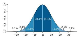
Normal Poisson distribution around the mean, where each band has a width of one standard deviation
