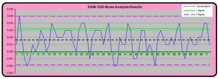
BAM-1020 Zero Test Analysis With 1.6µg Average, 1.7µg Hourly Standard Deviation, 3.4µg Hourly Detection Limit
