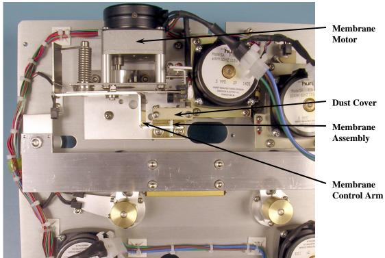
The Membrane Assembly Inside the BAM-1020
