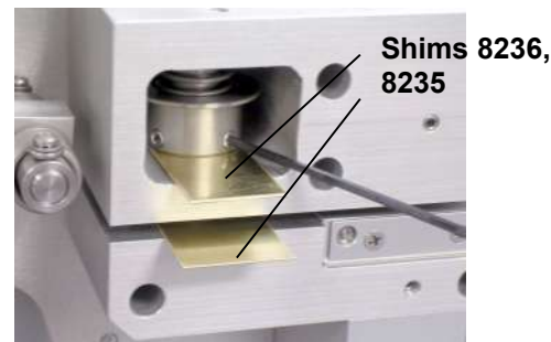
Using Shims for Reassembly
