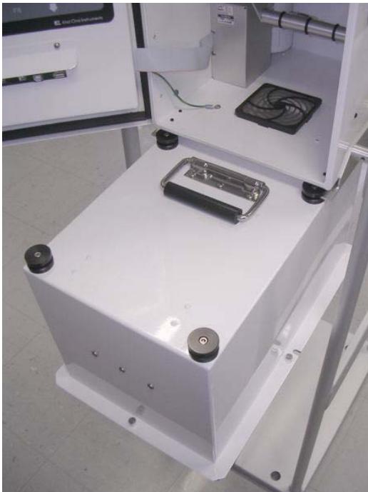
Figure 2-3 Pump Box Deploys by Sliding in to Rails Shown Here
