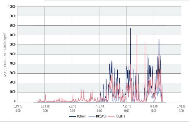
Source apportionment is the ability to tell whether the measured signal originates from the combustion of fossil fuels or from the combustion of biomass. When the outputs of the shorter wavelength channels on the BC 1054 (370-470nm) are higher than the outputs of the longer wavelength channels (525 – 950 nm) it usually signals the presence of organic compounds (sometimes called Brown Carbon "BrC"). The same is true when the 370 nm output of the BC 1060 is greater than 880 nm output.
