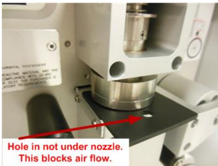
Figure 5-3 Nozzle Sealing Tool Lower System Test Configuration
