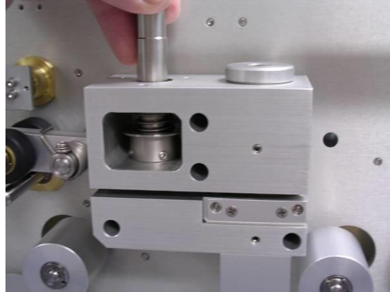
Removing the nozzle
