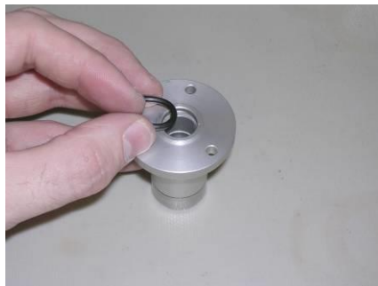
Replacing the nozzle o-ring
