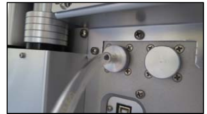
Figure 6-11 Zero Calibrate Screen and Sheath Air Pre-Filter Inlet Tubing Installation
