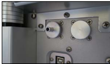
Figure 6-11 Zero Calibrate Screen and Sheath Air Pre-Filter Inlet Tubing Installation
