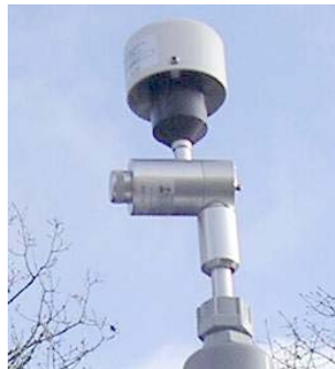
Figure 2-1 Sharp cut cyclone attached to intake
