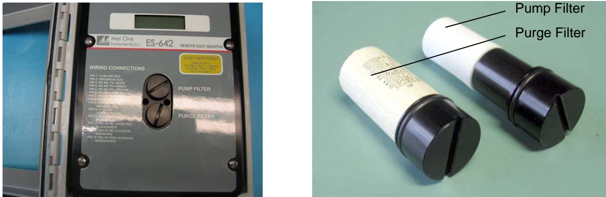
Figure 6-1 Pump Filter and Purge Filter Replacement
