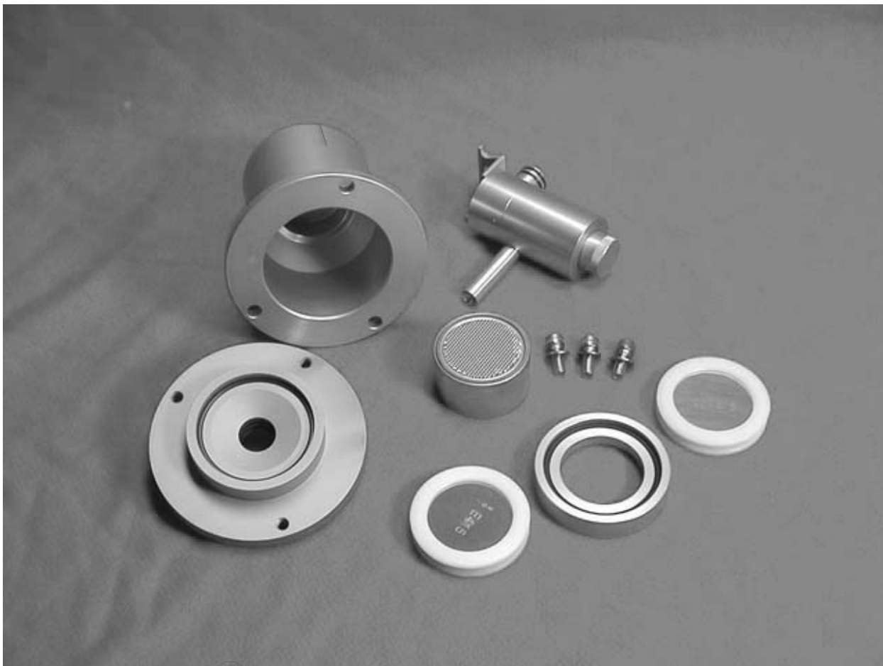
Figure 1.4 Photograph of the disassembled SASS Canister, showing the SCC Inlet, the MgO denuder, the front and back filters and the protective canister.
