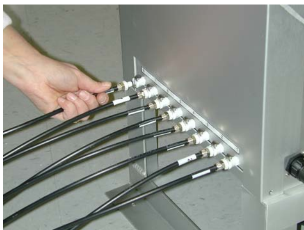
Figure 2.10 Tubing Installation (SuperSASS)
