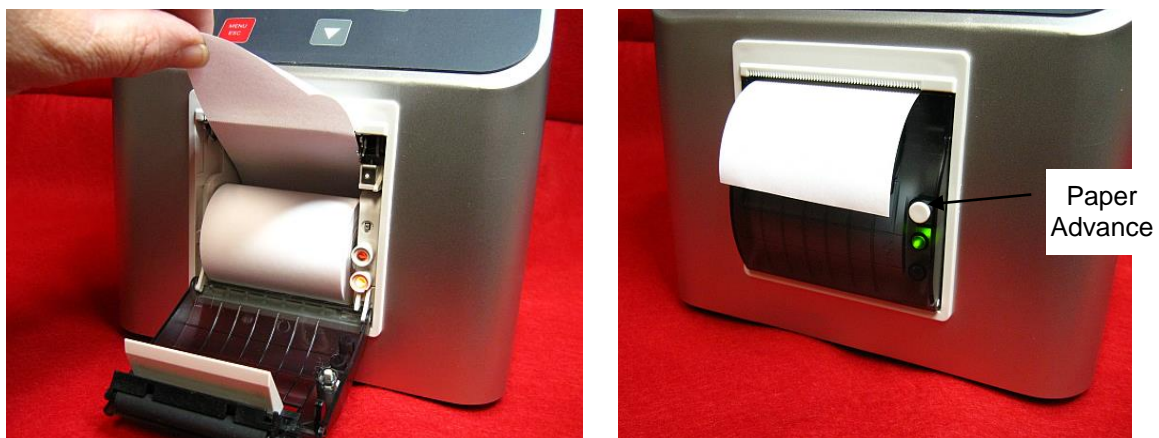
Figure 6 – Install Paper and Close Printer Door
