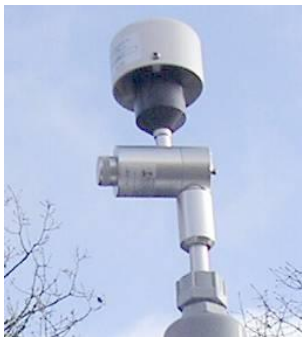
Figure 2-1 Sharp cut cyclone attached to intake
