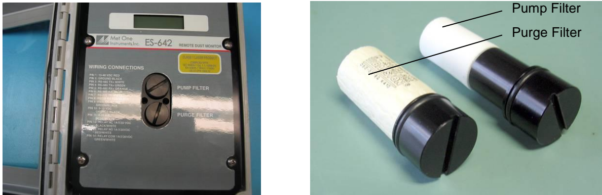
Figure 6-1 Pump Filter and Purge Filter Replacement
