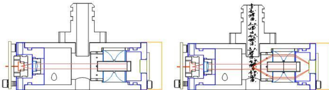
Figure 8-2 MDF Clean Air and Particulate Scatter Conditions in the MD Engine
