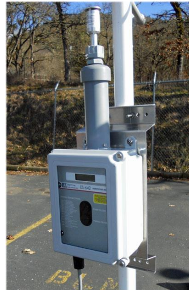
Figure 2-4 Typical Pole Mounting
