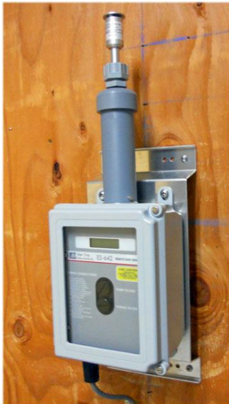
Figure 2-3 Typical Wall Mounting
