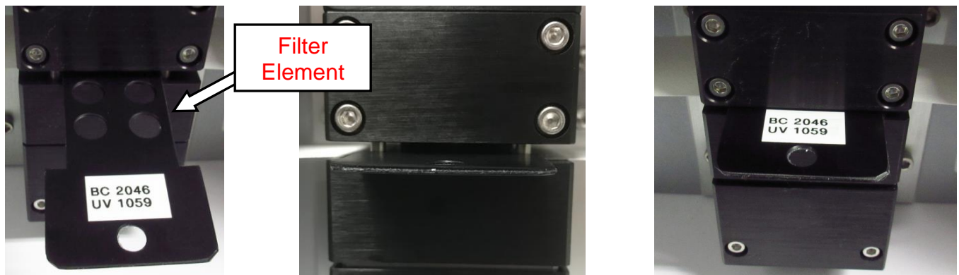
Figure 6-13 Inserting the Neutral Density Span Membrane
