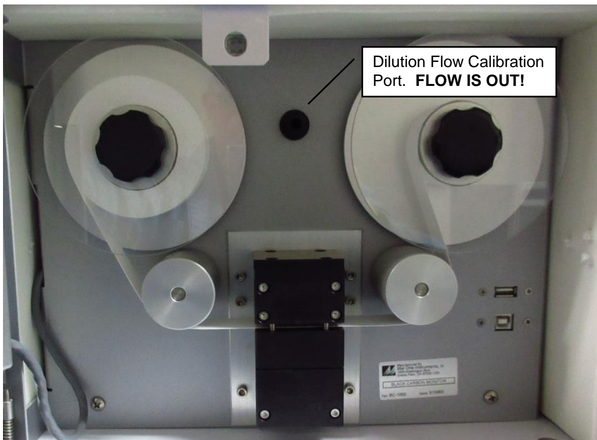
Figure 6-5 Dilution Flow System Calibration Port
