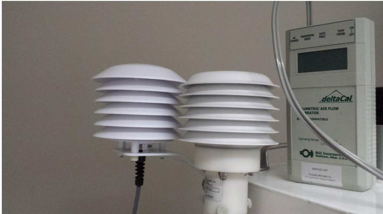
Figure 6-7 Ambient Temperature Audit with BX-307
