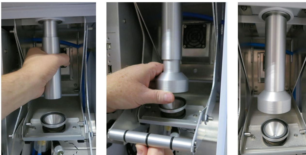
Figure 3-8 Installation of the PM 10 Pass-Through Adapter
