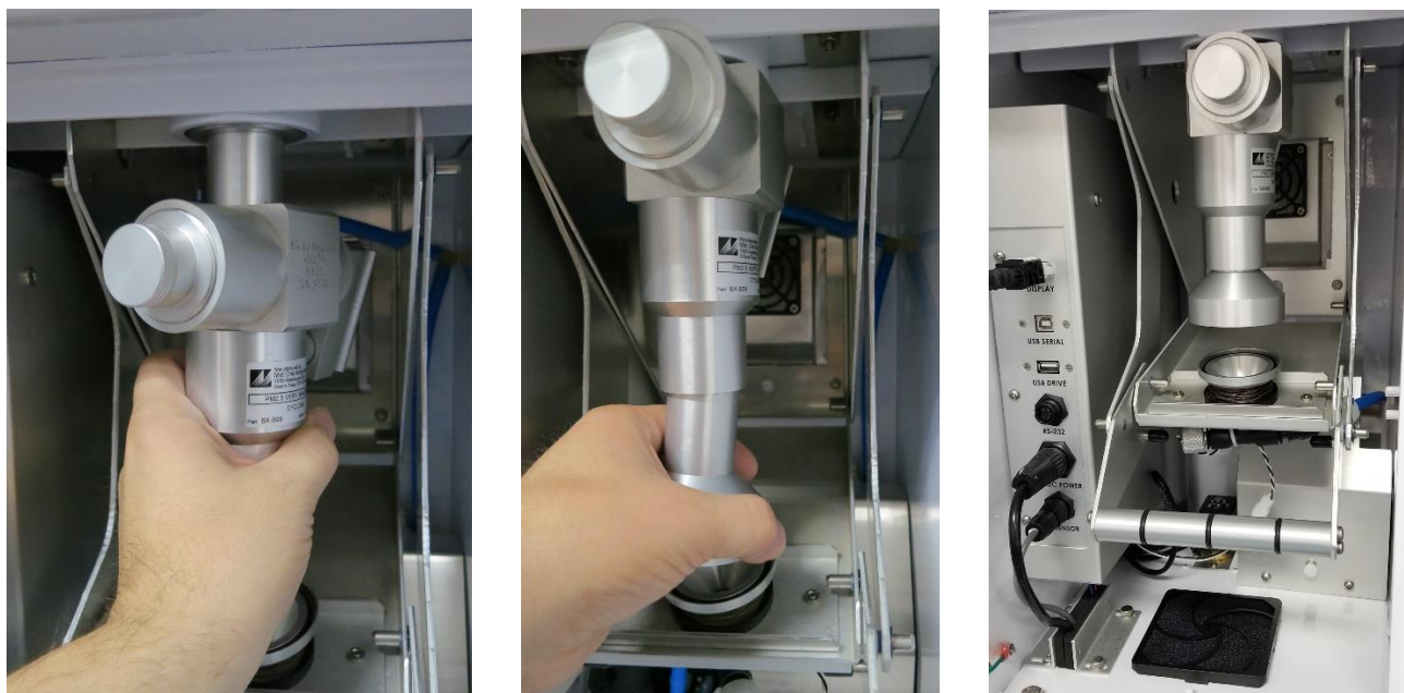
Figure 3-7 Installation of the PM 2.5 Cyclonic Separator
