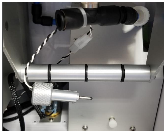
Figure 6-9 Filter Temperature Sensor Removed
