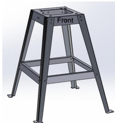
Figure 3-3 E-FRM-DC Sampler Stand Final Assembly
