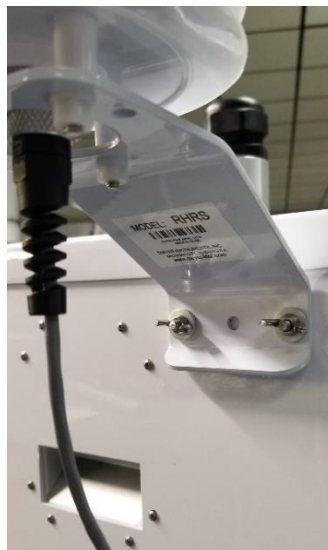
Figure 3-5 Ambient Temperature Sensor Assembly Mounting
