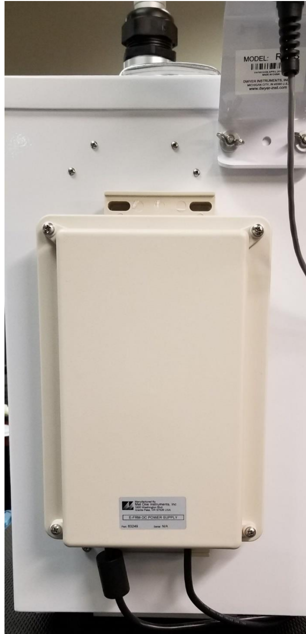
Figure 3-9 Securing the Power Supply Case
