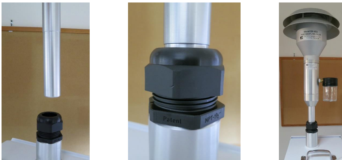
Figure 3-6 Installation of the PM 10 Inlet
