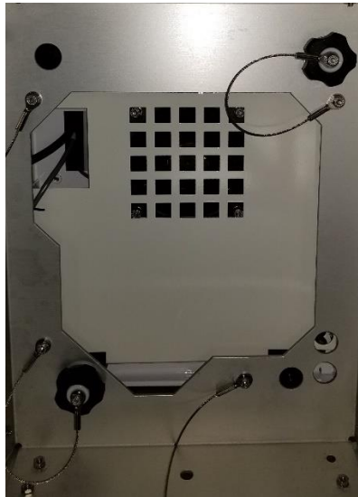
Figure 3-4 Securing the E-FRM-DC Sampler to the Stand
