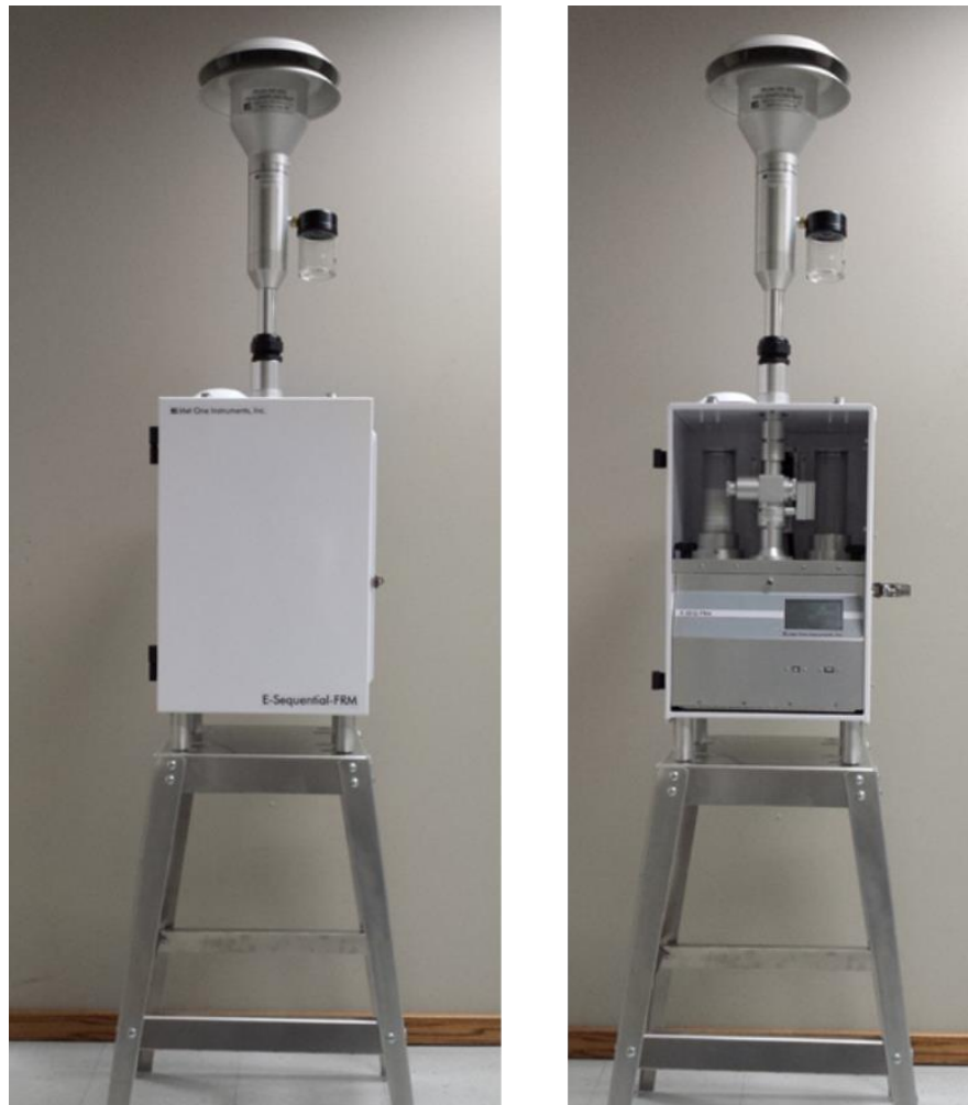
Figure 3-2 E-SEQ-FRM front views with and without door
