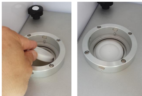
Figure 7-8 Inserting the Internal Leak Test Cassette
