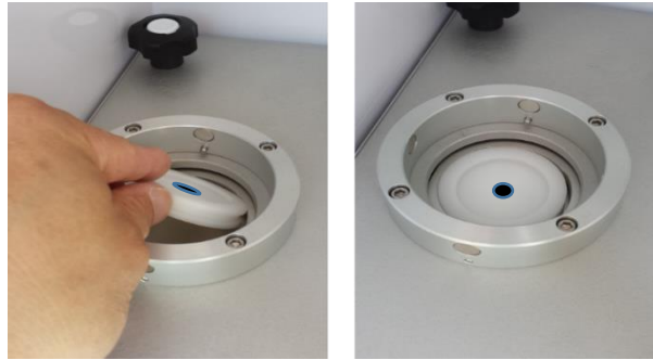
Figure 7-3 Inserting the External Leak Test Cassette
