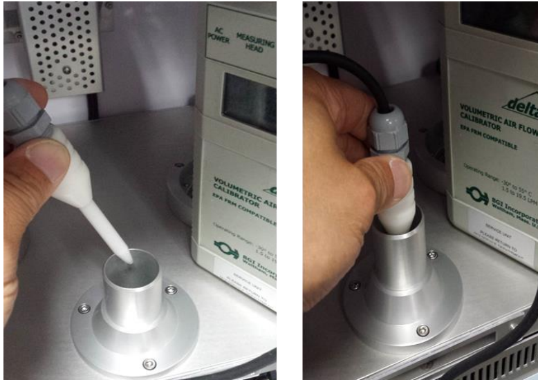
Figure 7-13 Filter Temperature Audit with BX-307
