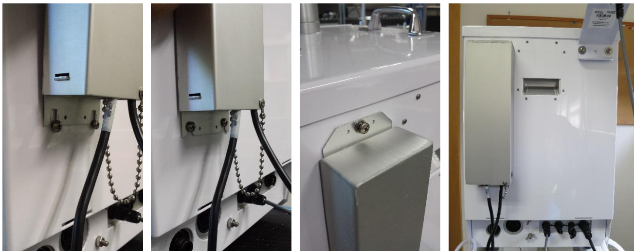
Figure 3-12 Securing the Power Supply Case
