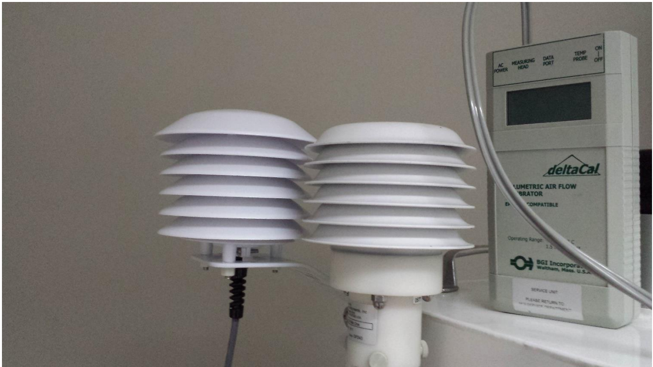
Figure 7-12 Ambient Temperature Audit with BX-307
