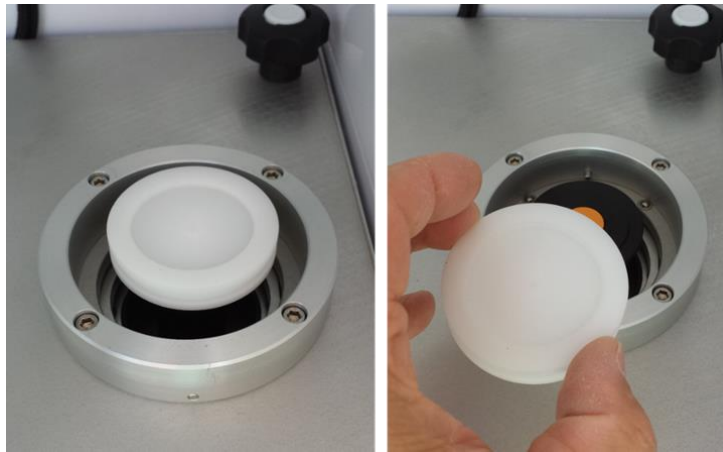
Figure 7-11 Removing the Internal Leak Test Cassette
