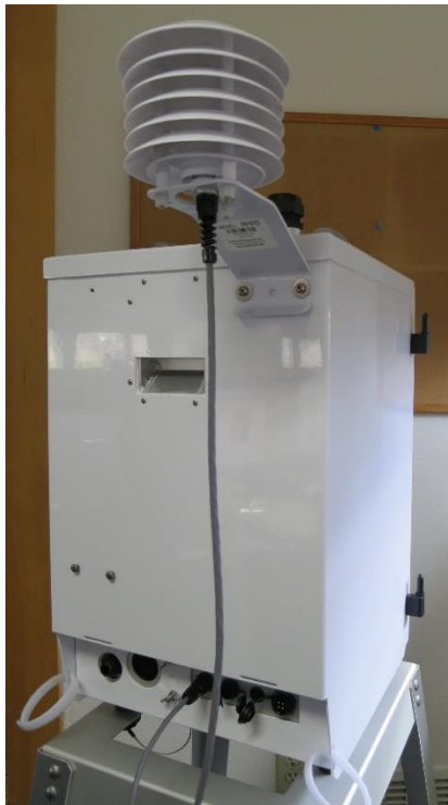
Figure 3-6 Ambient Temperature Sensor Assembly Mounted on the Enclosure
