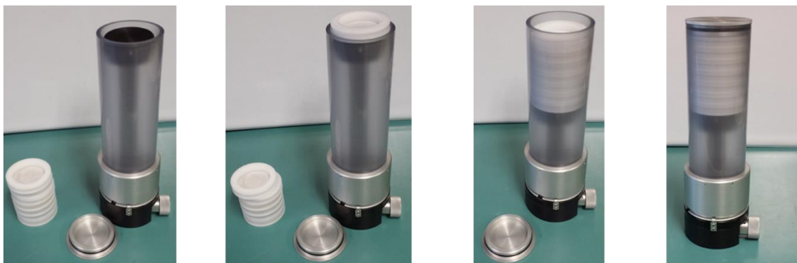
Figure 3-18 Loading New Filter Cassettes into the Magazine
