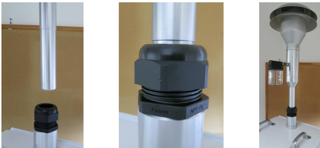
Figure 3-7 Installation of the PM 10 Inlet
