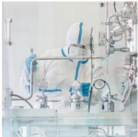
A cleanroom has a top to bottom laminar air flow at ISO Class 3 and below. These cleanrooms are normally on raised flooring such that air penetrates holes of the flooring. The idea is that any particles generated in the cleanroom are being pushed straight downwards such that they are flushed out through the raised flooring in the shortest possible path to contamination. This laminar flow of particle free air is generated via HEPA filters.
