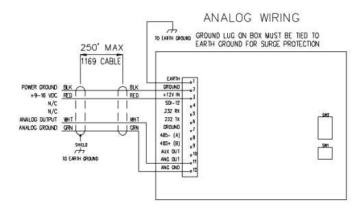
**Figure 3.1 – Analog Wiring**
