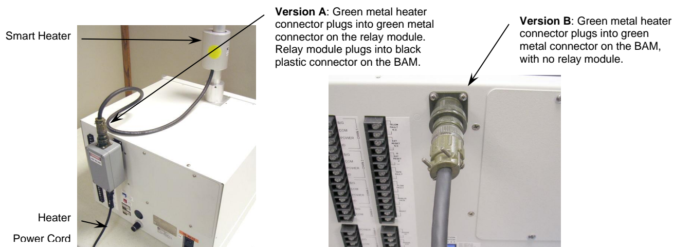
Two Different Smart Heater Power Configurations
