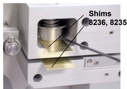
Using Shims for Reassembly
