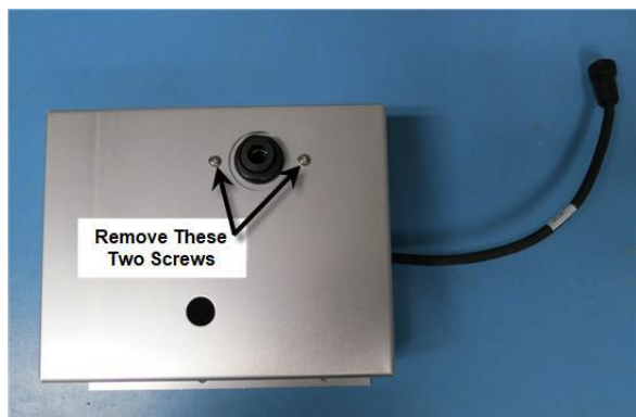
Figure 2-6 Dilution Flow System Cover Removal
