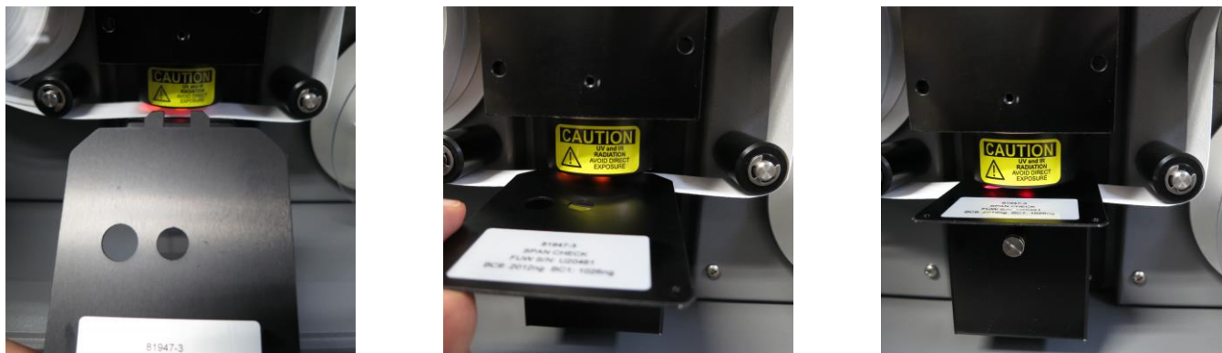
Figure 5-14 Inserting the Neutral Density Span Membrane
