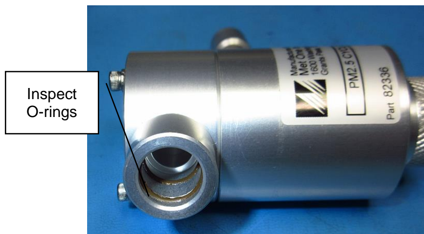
Figure 6-6 Unscrew and clean particle trap
