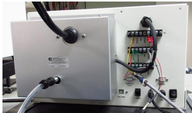
Figure 2-10 Dilution Flow System Installed
