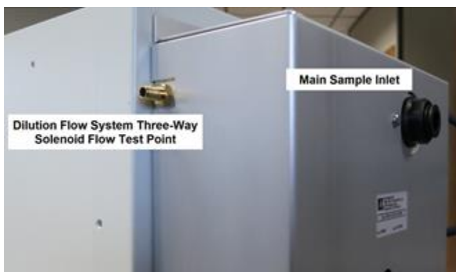
Figure 5-5 Dilution Flow System Air Flow Locations
