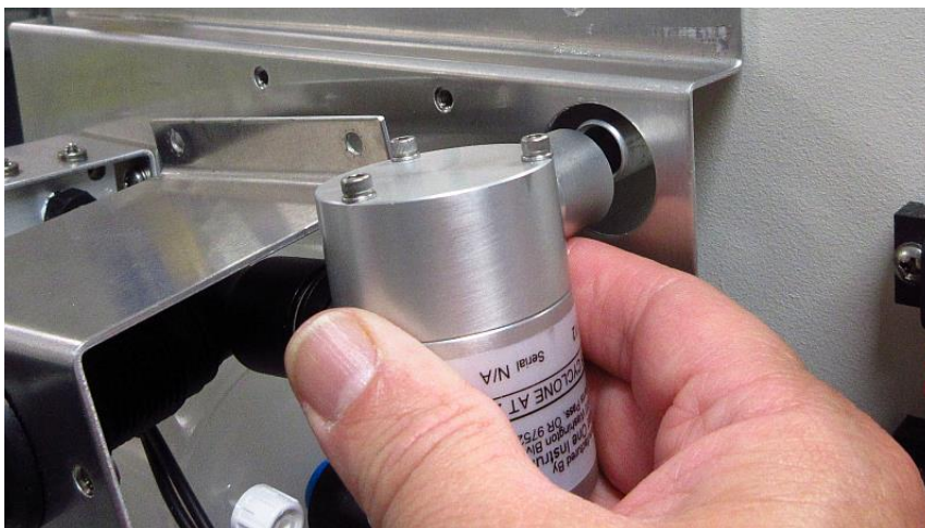
Figure 6-8 Pull cyclone away from BC 1054 inlet fitting
