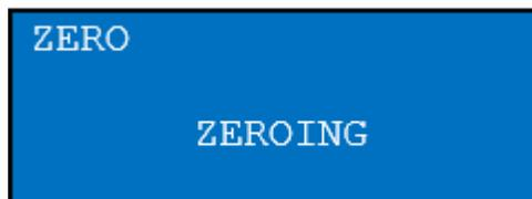
Once the zero calibration has finished, you will see the following screen below. Remove the Zero Filter Assembly and replace the sampling head. Press ESC to go back to the Service Menu.
