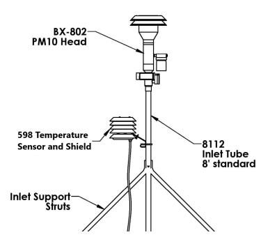
**Figure 1 Temperature Sensor Installation**
