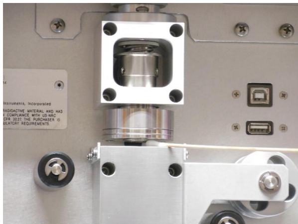
Figure 5-6 Cleaning the E-BAM Nozzle and Vane with a Cotton-Tipped Applicator
