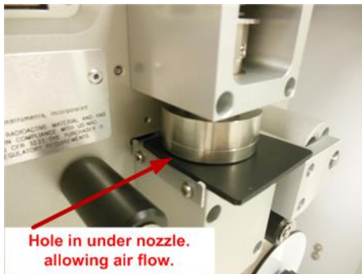
Figure 5-4 Nozzle Sealing Tool Upper System Test Configuration
