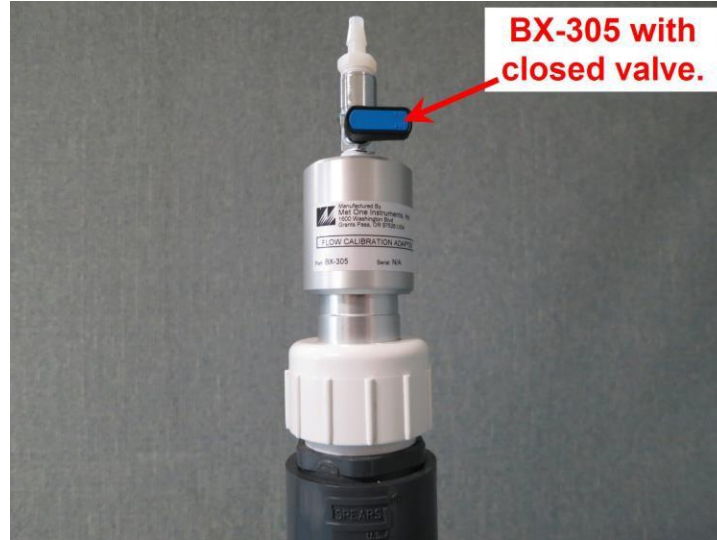
Figure 5-2 BX-305 Installed on Inlet Tube
