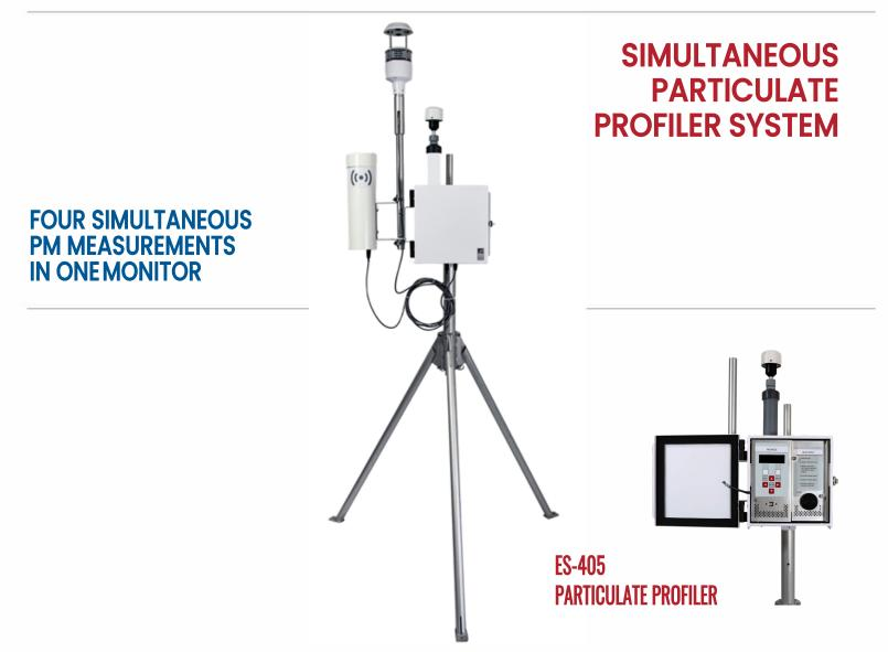
**Met One Instruments, Inc. AQ EAGLE is a system utilizing our ES-405 Particulate Profiler.** The ES-405 continuously samples ambient air and reports particulate mass concentrations simultaneously and in real time for PM<sub>10</sub>, PM<sub>4</sub>, PM<sub>2.5</sub> and PM<sub>1</sub>. Our ES-405 is ideal for fugitive emissions and neighborhood scale community monitoring projects where both simple operation, portability and modest cost of
