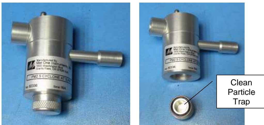
Figure 6-4 Unscrew and clean particle trap
