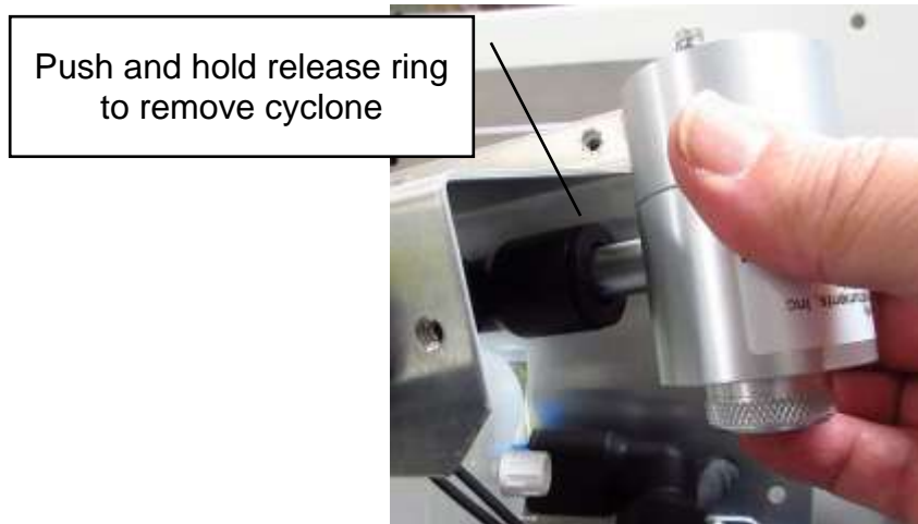
Figure 6-9 Push and hold release ring
