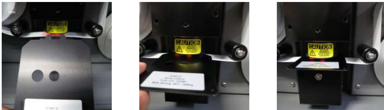
Figure 5-14 Inserting the Neutral Density Span Membrane
