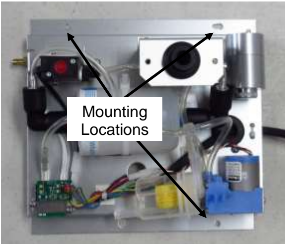
Figure 2-8 Dilution Flow System Mounting Screw Locations
