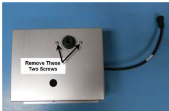
Figure 2-6 Dilution Flow System Cover Removal
