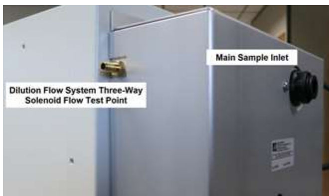
Figure 5-5 Dilution Flow System Air Flow Locations
