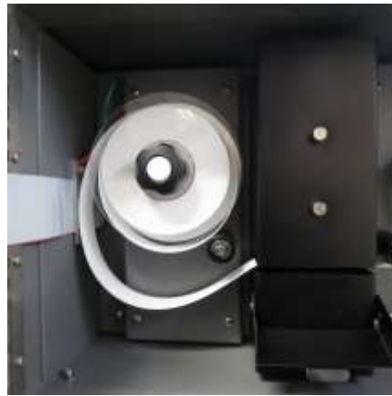
Figure 5-9 Loosening the Tape for Cover Removal
