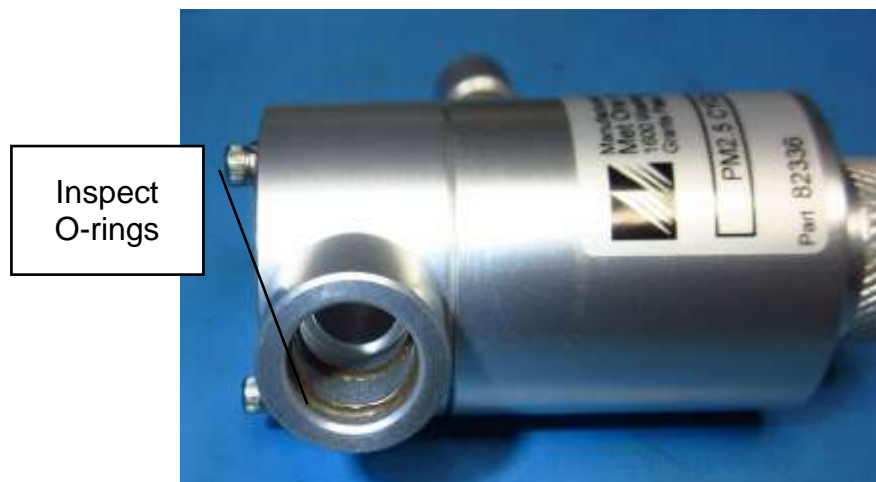
Figure 6-6 Unscrew and clean particle trap
