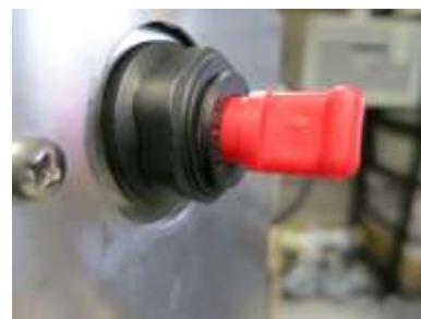
Figure 6-1 Leak Check Sealing Plug Installation
