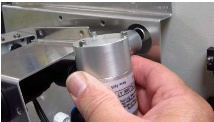
Figure 6-8 Pull cyclone away from BC 1054 inlet fitting
