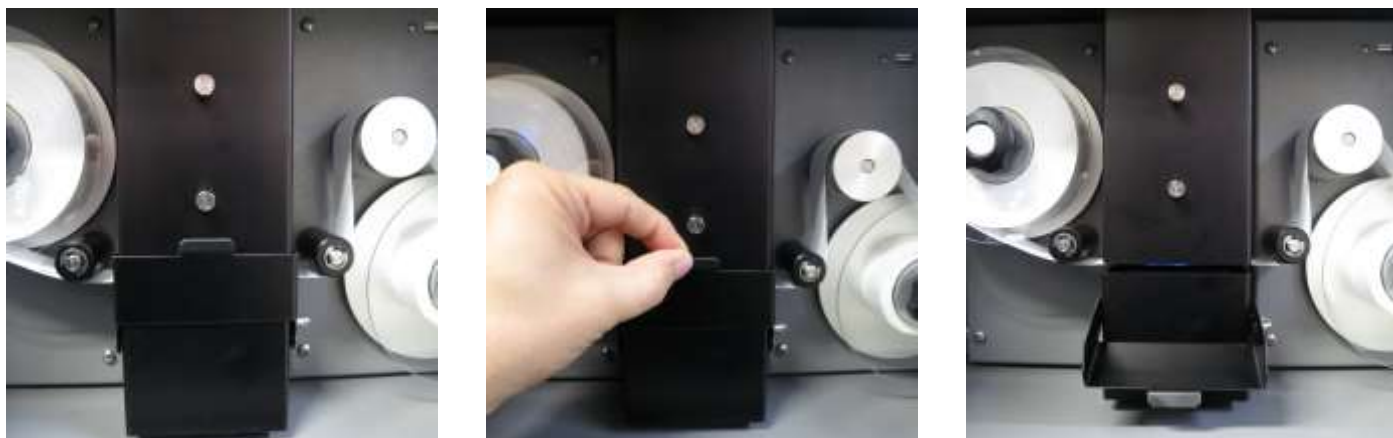
Figure 5-8 Opening the Tape Slot Access Door
