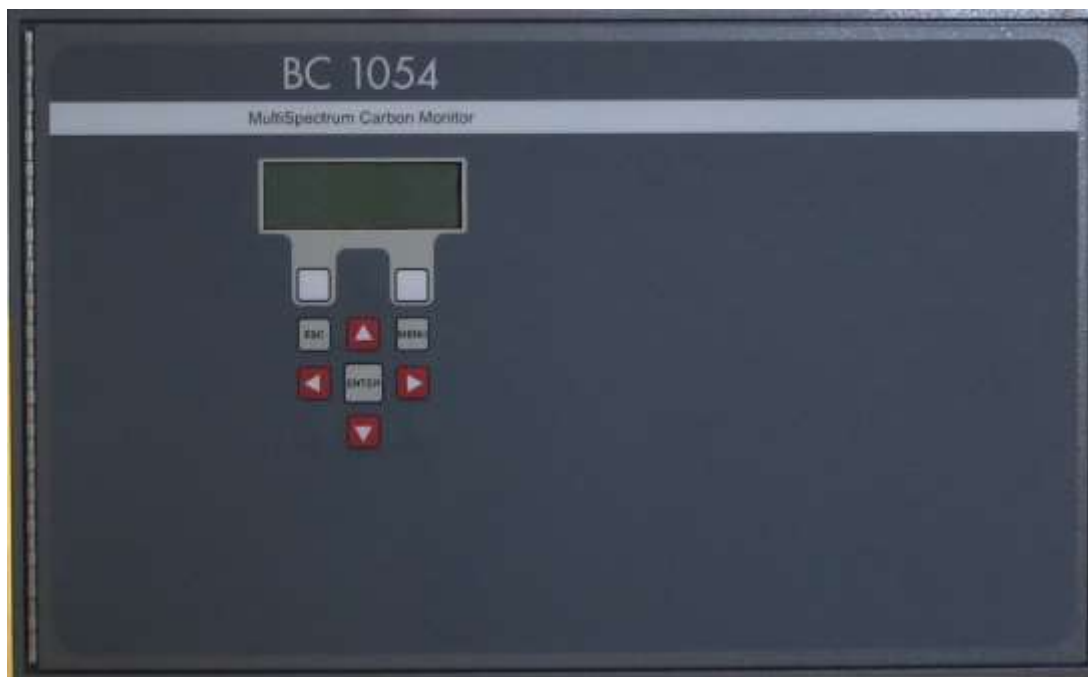
Figure 1-1 The BC 1054 Front Panel
