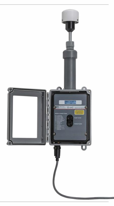
Measurement PrinciplesParticulate concentration by forward light scatter laser Nephelometer.Available Cut PointsTSP Inlet Standard. PM10, PM2.5, and PM1 sharp-cut cyclone inlets available.
