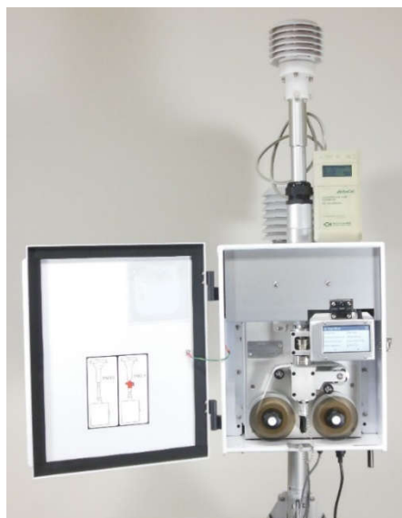
Figure 5-8 E-BAM with CTS Installed
