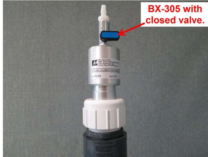
Figure 5-2 BX-305 Installed on Inlet Tube
