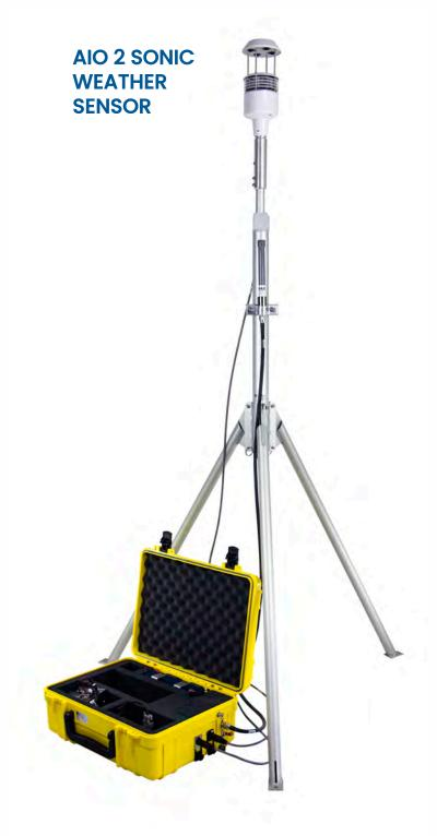
Power for the AIO 2 Sonic Weather Sensor and the rest of the remote site system components is provided from a commercially available, 8AH rechargeable battery. This battery, when fully charged, will operate the basic CAMEO/ ALOHA HAZMAT Weather Station system more than 5 days before requiring recharging or replacement. The basic system transit case holds the AIO 2 Sonic Weather Sensor, battery, radio transmitter, cables and other accessories.
