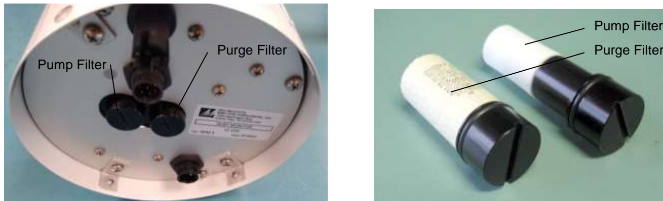
Figure 3 Pump Filter and Purge Filter Replacement
