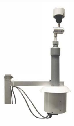
The NPM 3 is calibrated using 0.6µm NIST traceable polyspheres. These provide a critical and consistent baseline calibration. To correlate this calibration to real-world, non-spherical particulates, a Calibration Factor (K-Factor) is established by means of comparison to a collocated, trusted, and proven reference source (i.e., a BAM 1020) to ensure both accuracy and correlation.
