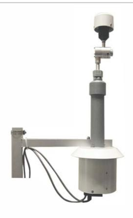
The NPM 3 is calibrated using 0.6-micron latex micro-spheres. These provide an extremely consistent calibration, but do not generally match the characteristics of all ambient particulate. A K Factor (multiplier) must be established, by using a collocated trusted reference source (such as a BAM 1020) for good accuracy and correlation. The default factory K Factor is 1.0.
