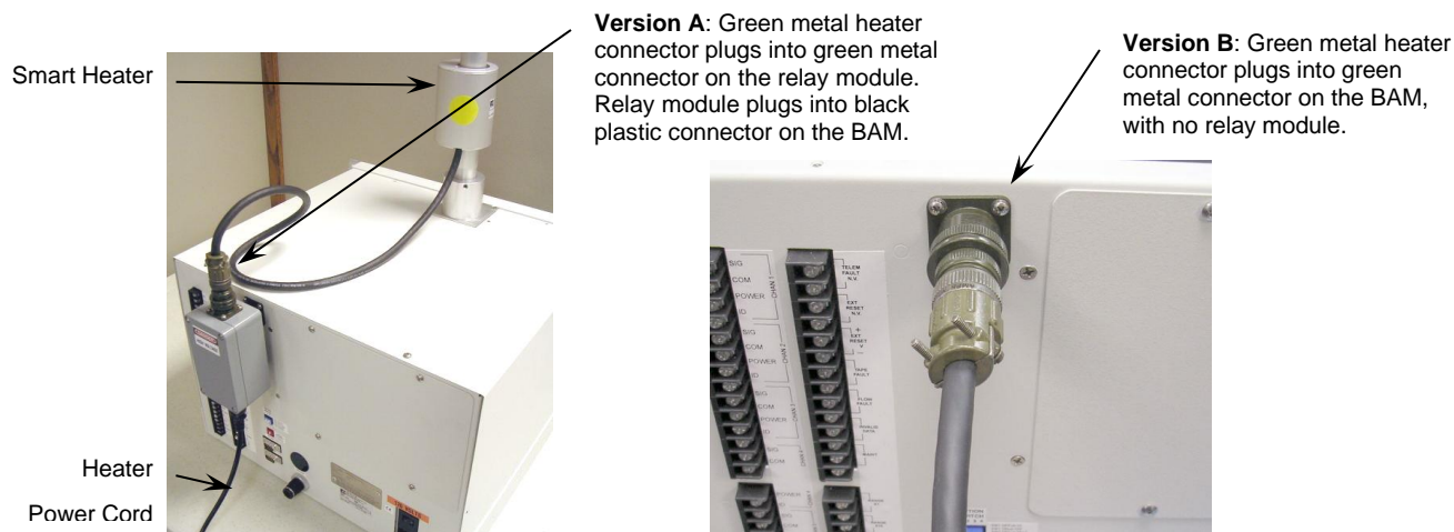
Two Different Smart Heater Power Configurations
