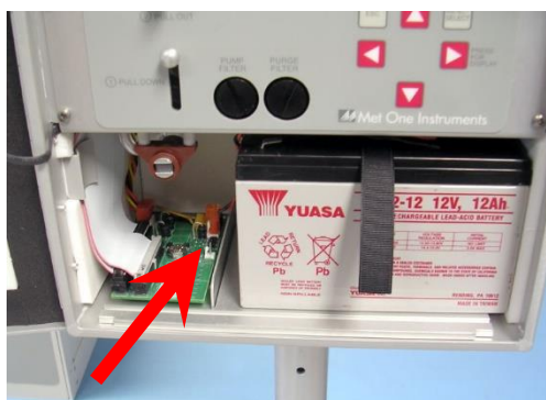
Internal battery and 81220 PCB battery harness connection
