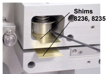
Using Shims for Reassembly
