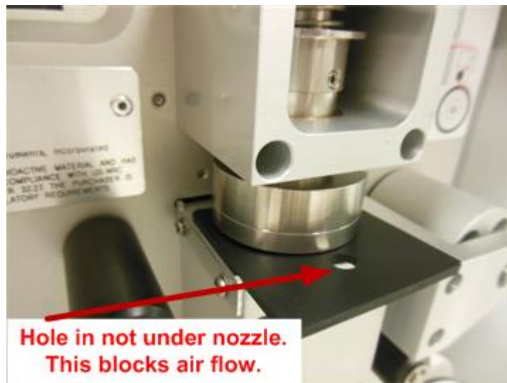
Figure 5-3 Nozzle Seal Tool with Solid Side Under the Nozzle
