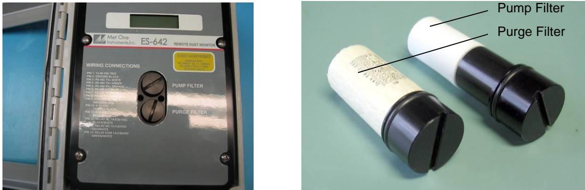
Figure 6-1 Pump Filter and Purge Filter Replacement
