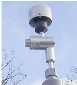
Figure 2-1 Sharp cut cyclone attached to intake
