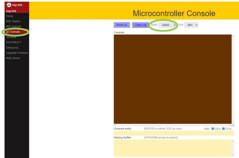
**Figure 7-5 - Microcontroller Console**
