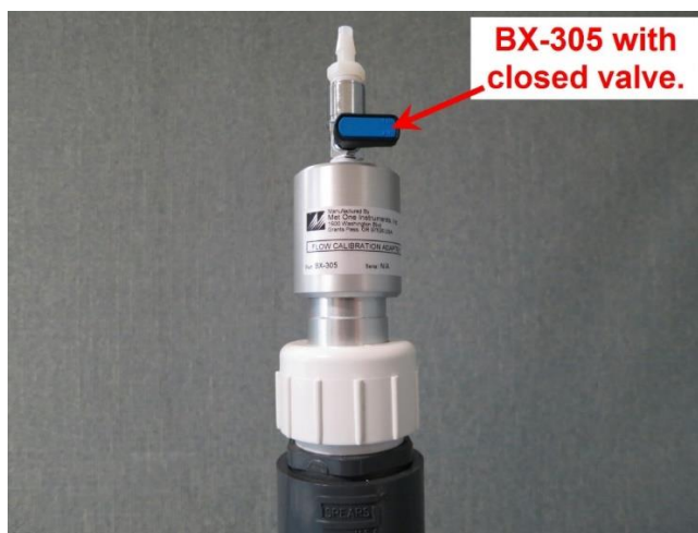
Figure 6-3 BX-305 Leak Check Valve Installed on Inlet Tube
