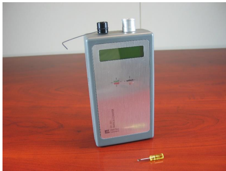
Figure 4 - Removing the Inlet Adapter seal
