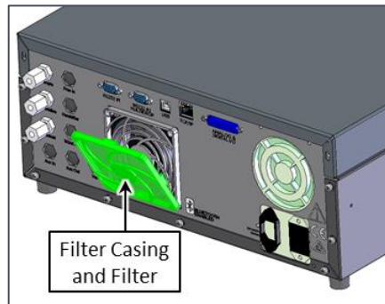
Figure 121 – Remove Filter Casing and Filter
