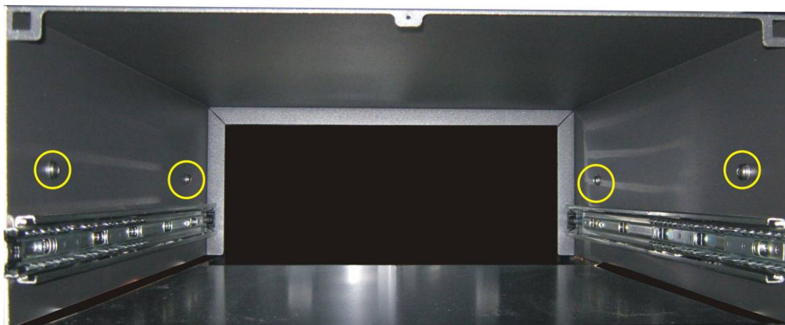
Figure 26 Installation of lid to rack mount brackets
