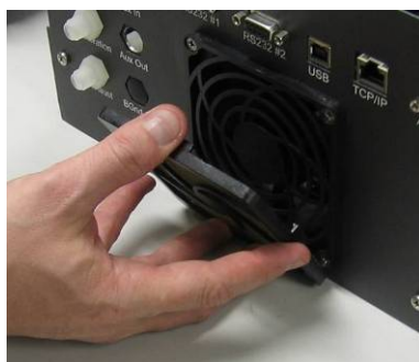
Figure 19 Removing fan filter
