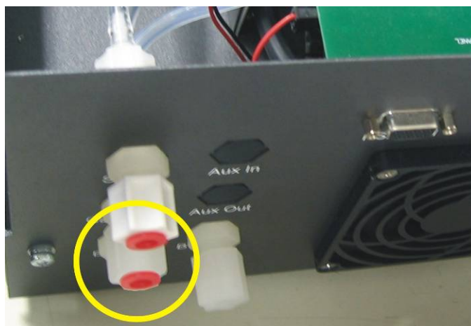
Figure 20 Plugged sample and calibration ports
