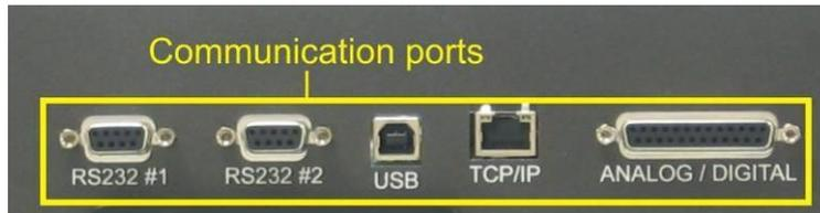
Figure 11 Communication ports
