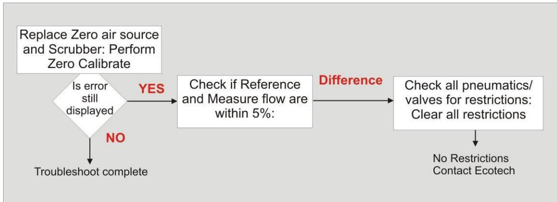
**7.3 TRS reaction cell temperature failure**
