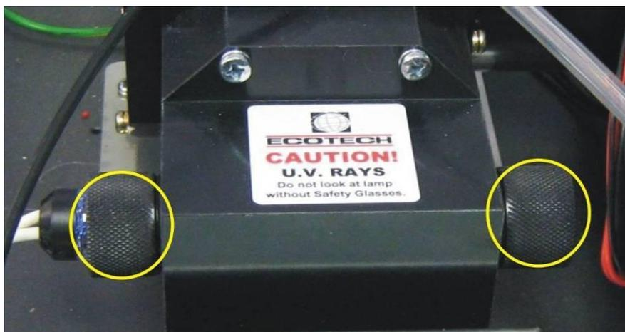
**Figure 27 Collets of the UV lamp**
