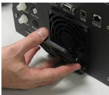
Figure 23 Removing fan filter
