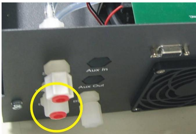
**Figure 24 Plugged sample and calibration ports**
