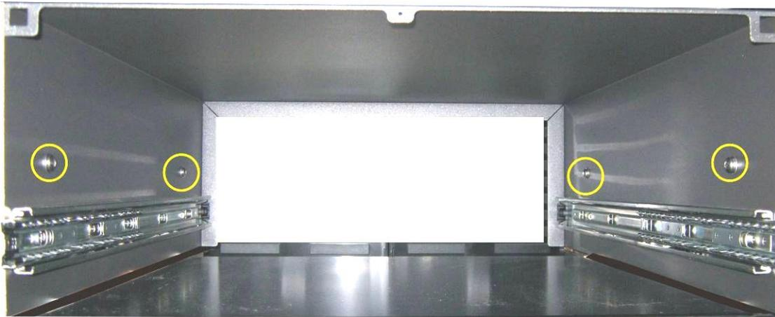
**Figure 30 Installation of lid to rack mount brackets**
