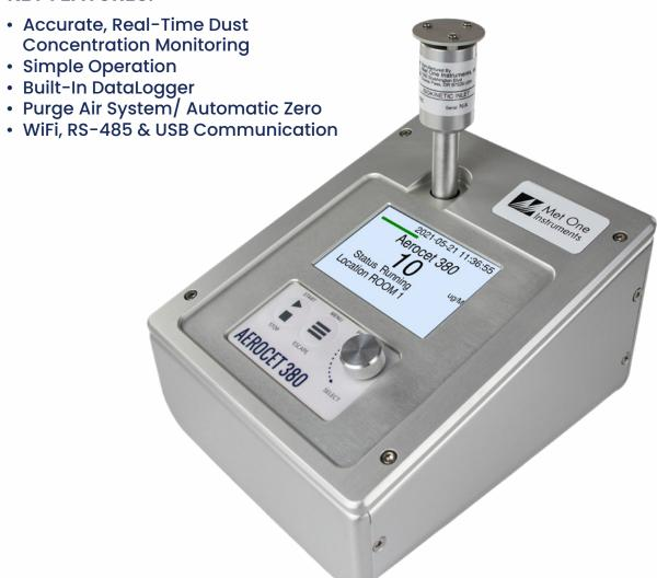
The Met One Instruments, Inc Aerocet 380 is a nephelometer that offers real-time airborne TSP (total suspended particulate) concentration levels using the principle of forward laser light scatter. This instrument is ideal for sampling in any indoor workplace or public place environment with optional separators to monitor PM<sub>1</sub>, PM<sub>2.5</sub>, or PM<sub>10</sub>.
