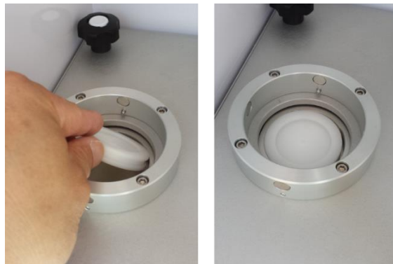
Figure 7-8 Inserting the Internal Leak Test Cassette
