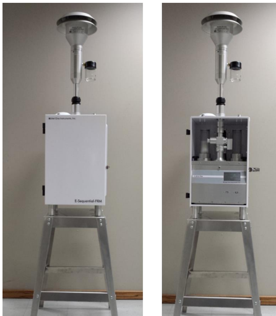
Figure 3-2 E-SEQ-FRM front views with and without door
