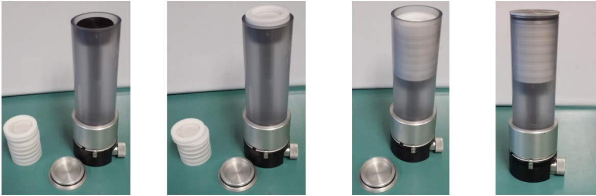
Figure 3-18 Loading New Filter Cassettes into the Magazine
