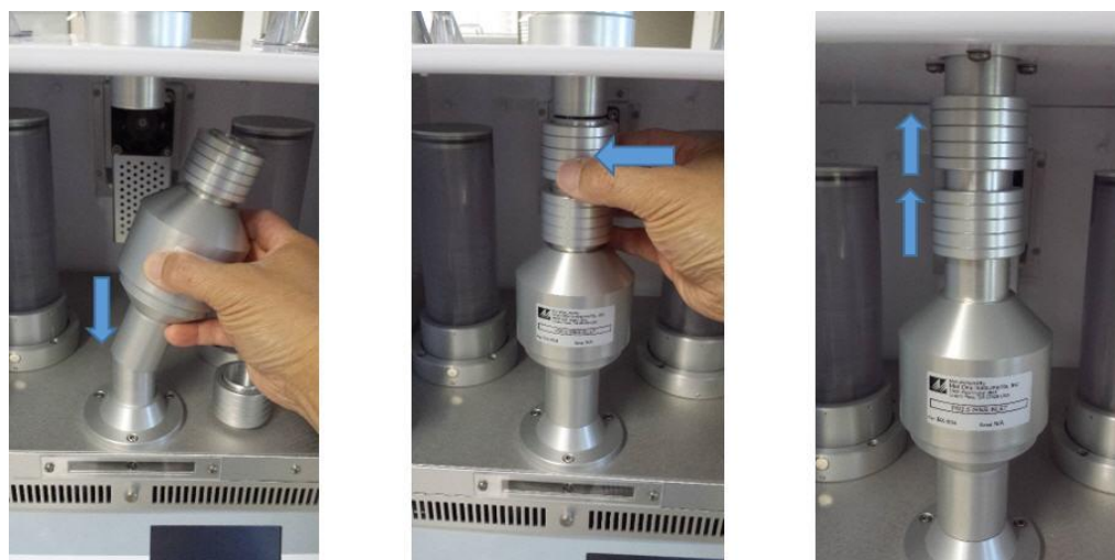
Figure 3-9 Installation of the PM 2.5 WINS Impactor
