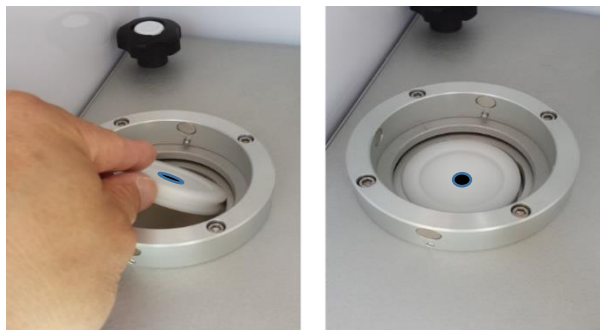
Figure 7-3 Inserting the External Leak Test Cassette
