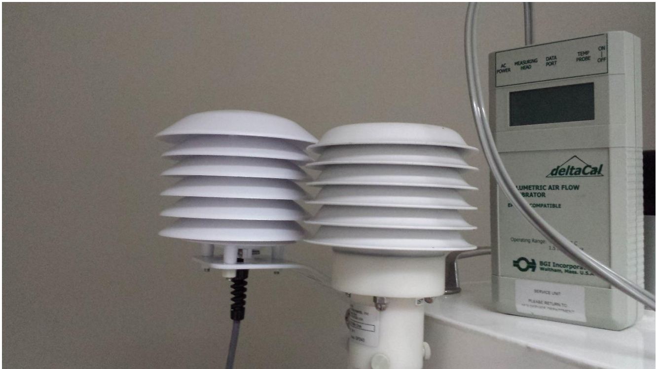
Figure 7-12 Ambient Temperature Audit with BX-307
